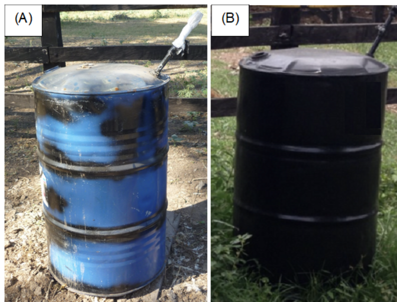
Figure 2. Anaerobic biodigester: (A) biodigester without black paint; (B) biodigester with black paint.
