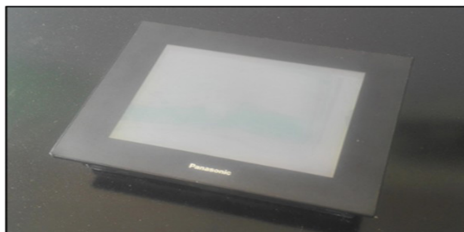
Fig. 18. Touch screen HMI display, Panasonic GT32M
