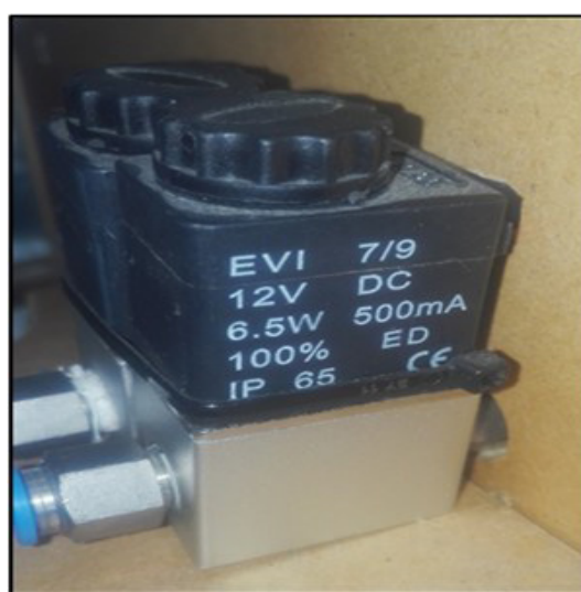
Fig. 6. Solenoid valves 12V DC
