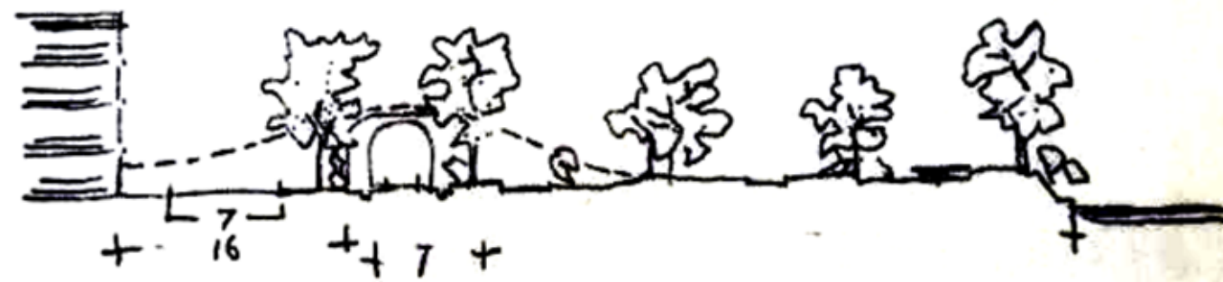
Figure 20. Elevation of pedestrian paths in sections where pedestrian flow is interrupted by railway lines. Source: (ICTA, 1950, p.3).
